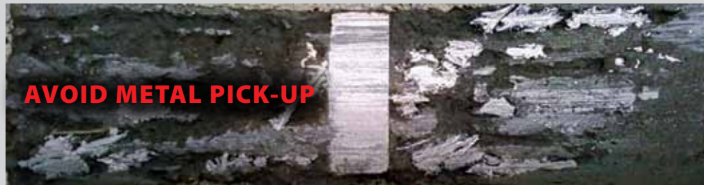
BEFORE: Large surface defect like the one shown on the R2 wheel increases kip-forces, causing track and wheel damage.
