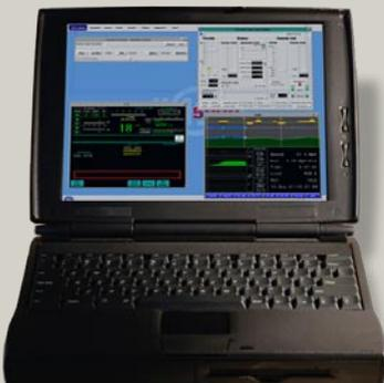
*Real-time data display shows in-train forces, brake pressure, train's position, and operating parameters.*
