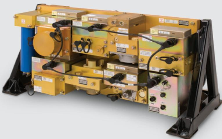
*The electro-pneumatic control unit (above) responds to the engineer's handle movements on the electronic brake valve, EBV.*
