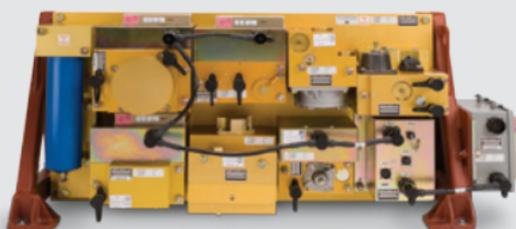
CCB-26, the low-cost, highly reliable replacement for 26L, is especially suited for new low-horsepower, low-emissions switcher locomotives or to upgrade existing locomotives.
