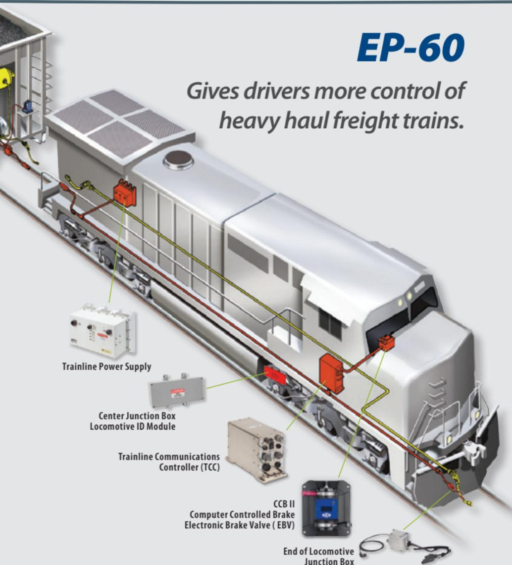
The EP-60 electronically controlled pneumatic brake (ECP) system dramatically reduces in-train forces and benefits you in three important ways.
